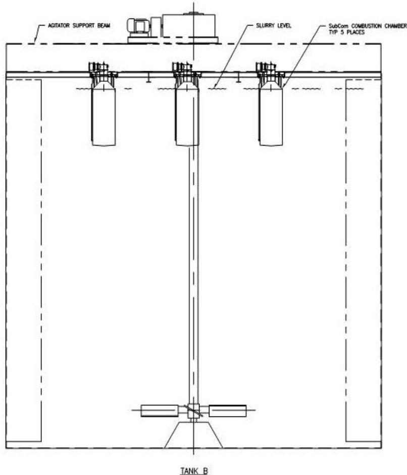
**Figure 3 – Slurry Storage Tank Heater Elevation Layout**
