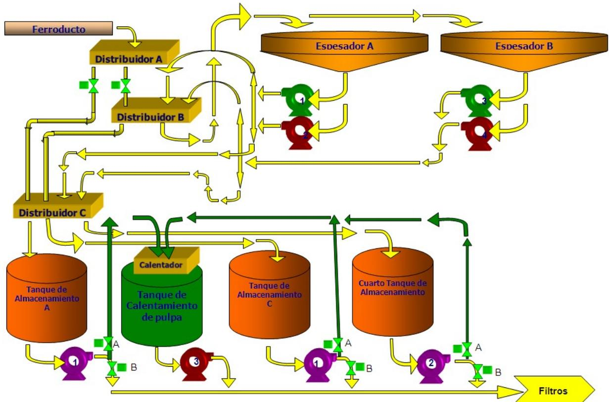
**Figure 2 – Iron Ore Processing Flow Diagram**
