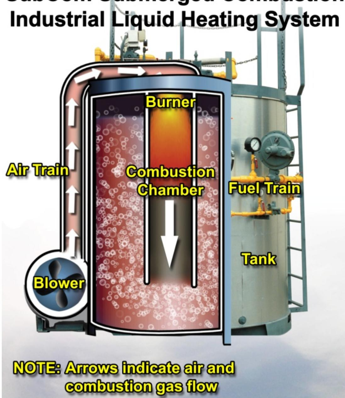
Figure 1 – SubCom Cutaway
