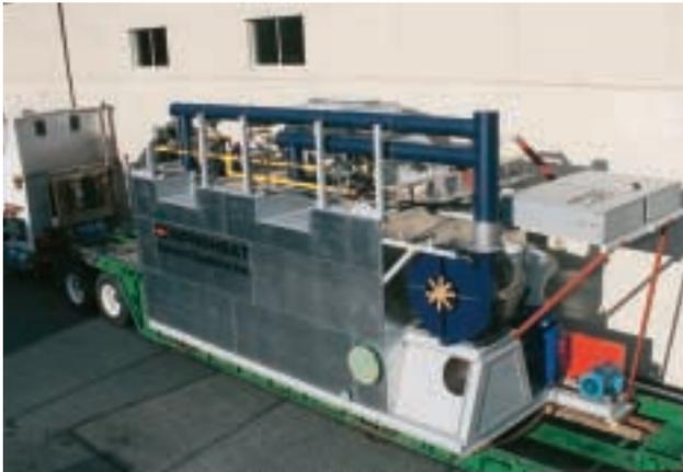
used to heat a continuous 120 USGPM flow of water by 30°F with a stack temperature of 67°F. The resulting overall system efficiency is calculated at 98.4%.
