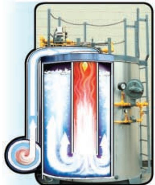
The use of submerged combustion technology in a variety of industries to replace traditional but inefficient methods of industrial liquid heating is helping to reduce CO<sub>2</sub> and heat emissions to the atmosphere. Photo shows a SubCom™ system recently installed at Konica's manufacturing plant in Whitsett, North Carolina.
